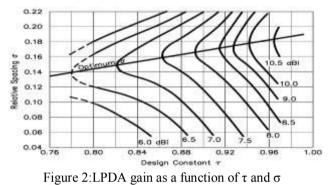
Step 1: Using Figure (1), find  $\tau$  and the figure(2) is labeled by gain .Determine the curve corresponding to the desired gain G and find its intersection with the straight line.
