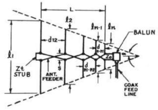
Figure 1: Log Periodic Dipole Antenna
