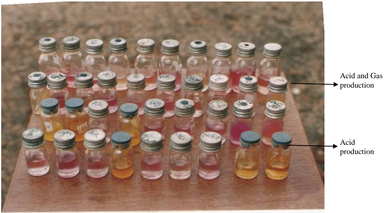
Plate IV. Biochemical tests including sugar fermentation, acid and gas production
