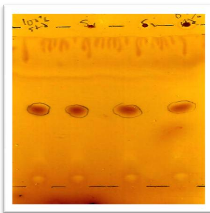
Figure. 1: TLC of Reference Chloroquine and formulated samples (RF=0.423)
