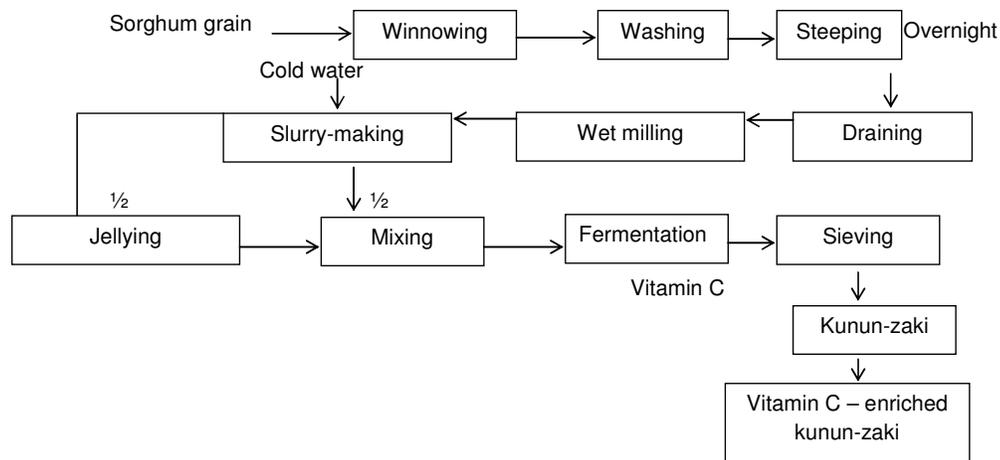
**Figure 1.** The modified laboratory method of kunun-zaki production (Egbere et al, 2008).
